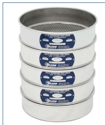
Figure 2. Test sieves. Image courtesy Gilson Company, Inc.
