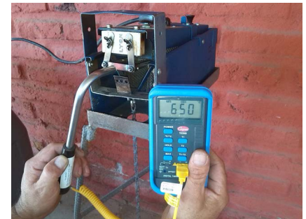
Pyrometer indicating proper blade temperature of 650°C.
